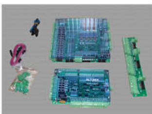
Elevator Control Card
